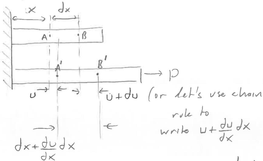
$$\epsilon_x = \frac{\Delta L}{L} = \frac{A'B' - AB}{AB} = \frac{x + \frac{du}{dx} dx - x}{dx} = \frac{\partial u}{\partial x}$$
