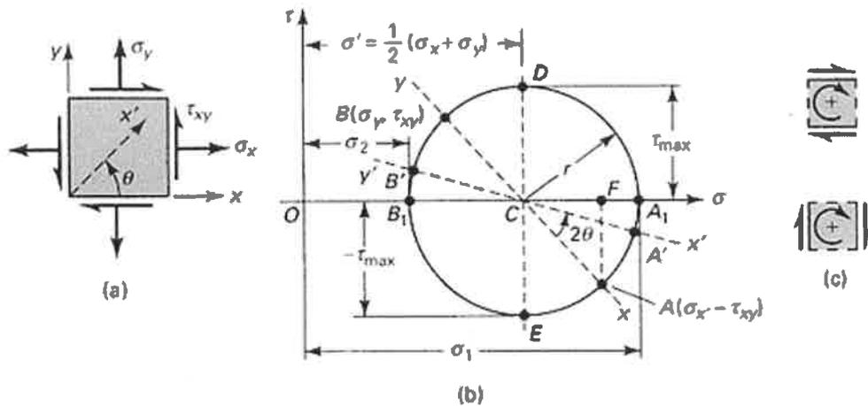
Given  $\sigma_x$ ,  $\sigma_y$ , and  $\tau_{xy}$  with algebraic sign in accordance with the foregoing sign convention, the procedure for obtaining Mohr's circle (Figure above) is as follows:
